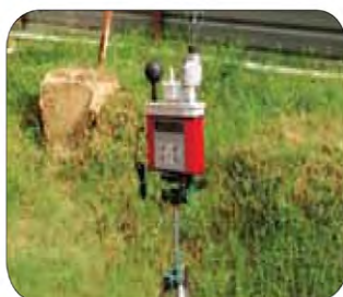
Figure 7: WGBT Monitor (Including Globe thermometer)
